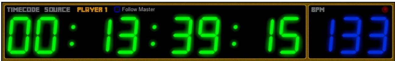
The above display shows the output time code and BPM information from the selected source, in this case “Player 1”. The “Follow Master” check box instructs TimeLord to follow the Master player in the PDJ network, as controlled by the DJ. Disable this to manually follow a specific player using the “Follow” button shown on the player windows.
