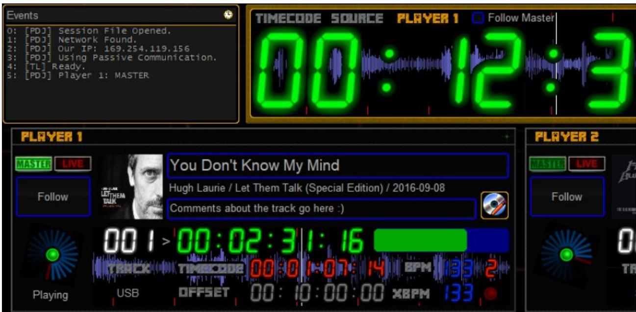
It's possible to get the waveform to display under the players time code display, such as shown above. To do this, you will need to edit the C:\Users\Public\TimeLord\TimeLord.ini file and change the line "PRODJ\_WAVEFORMUNDERPLAYER = 0" to read "PRODJ\_WAVEFORMUNDERPLAYER = 1"
